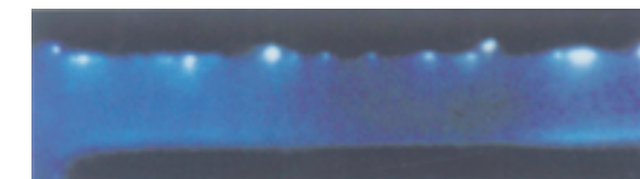
When interrupted, a concentrated electric arc ( I=40\text{kA} , transverse magnetic field contact) is generated.
